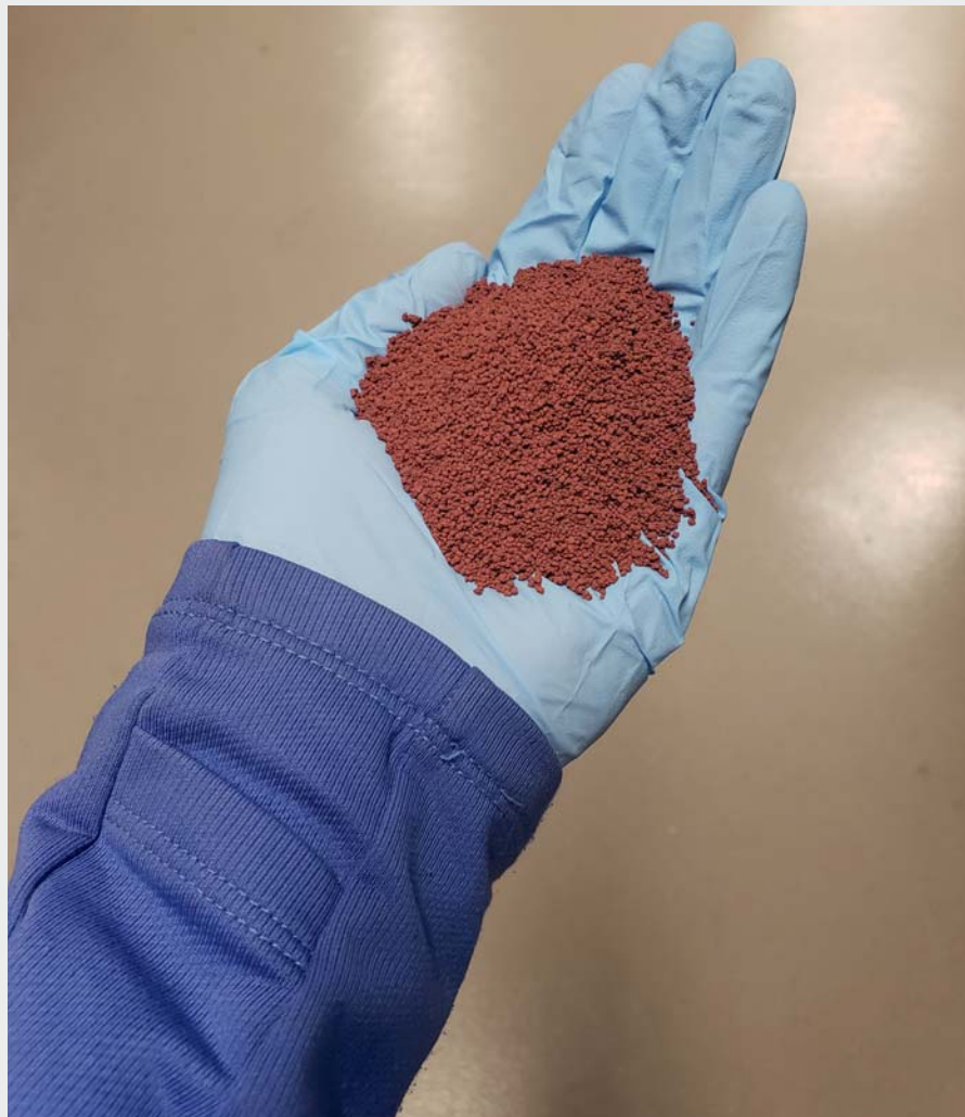
The active material, an iron- and aluminum-based metal oxide.
